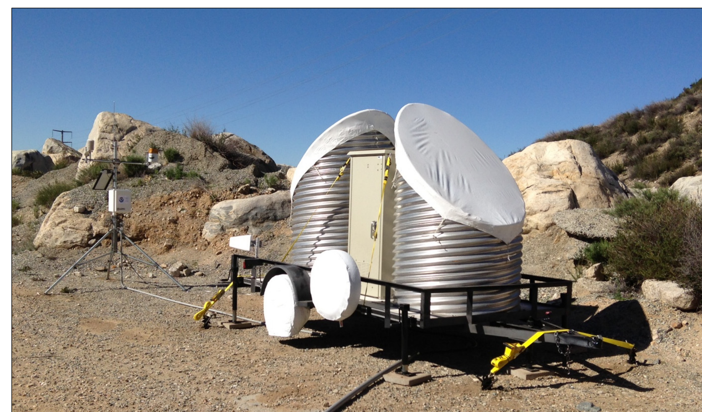
Figure 2. The NOAA S-band frequency-modulated, continuous-wave Doppler radar (SLR) at San Bernardino, California (SBO; see map). The shelter houses the radar hardware and data communications computer. An example of SRL data is shown in Figure 4.
