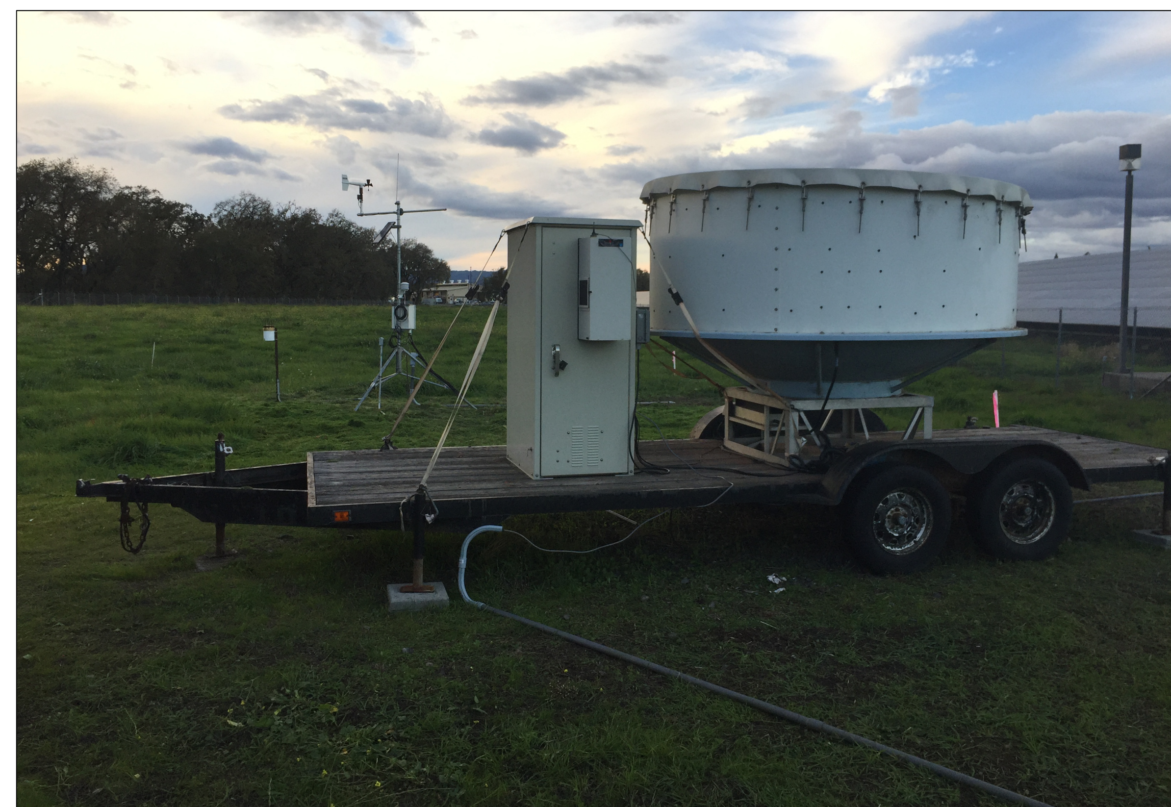
Figure 1. The NOAA S-band precipitation profiling Doppler radar (S-PROF) at Santa Rosa, California (STR; see map). The shelter houses the radar hardware and data communications computer. An example of S-PROF data is shown in Figure 3.
