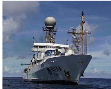
The C-band weather radar atop the central mast of the Ronald H. Brown research vessel.
