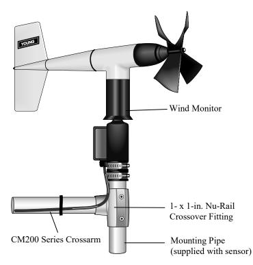
FIGURE 7-2. Wind monitor mounted to a crossarm by using 1- x 1-in. Nu-Rail Crossover Fitting
