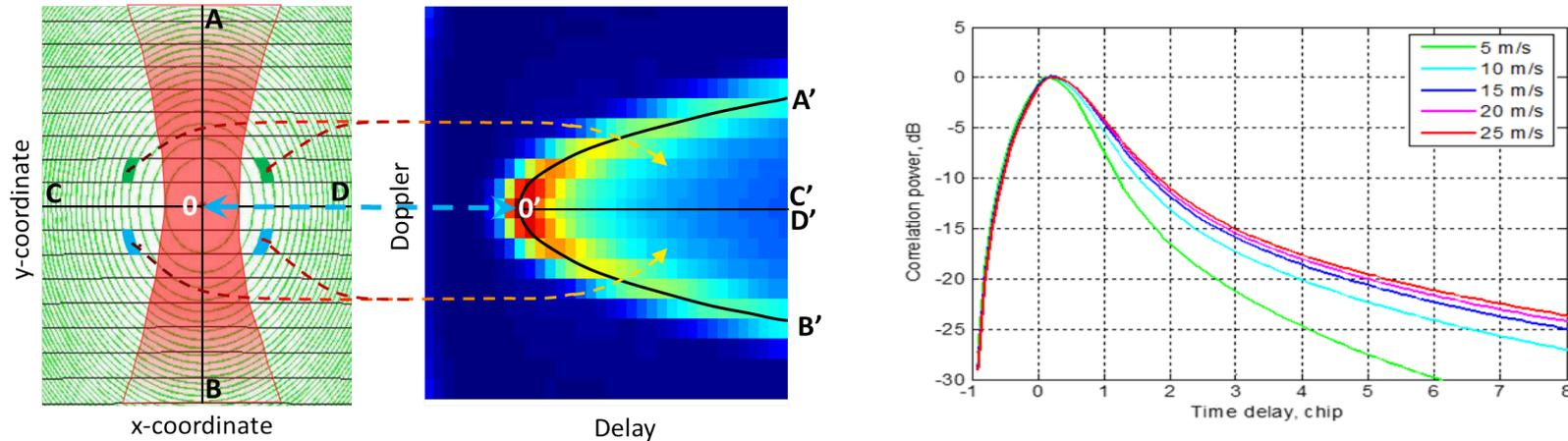
Delay-Doppler map emerges as a convolution of the Woodward Ambiguity Function with the Bistatic Radar Cross Section function within the antenna footprint described by its gain pattern. In a sense, delay-Doppler mapping creates an image of the scattering coefficient in the delay-Doppler domain:
