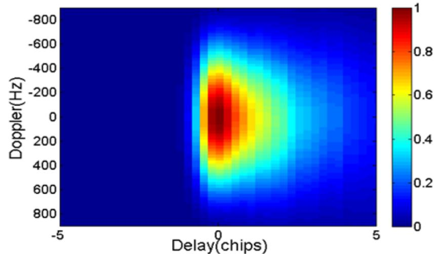
Delay-Doppler Mapping (DDM) creates an image of the scattering coefficient of the surface roughness in the delay-Doppler domain similar to Synthetic Aperture Radar.
