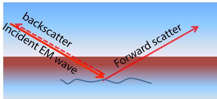
Benefits: (1) the transmitter is already out there, for free; (2) the receiver has a small form factor, a low power consumption; (3) forward scattering differs from backscattering and provides plenty of signal compared to monostatic radar; (4) less rain/snow attenuation compared to X and K-band.
