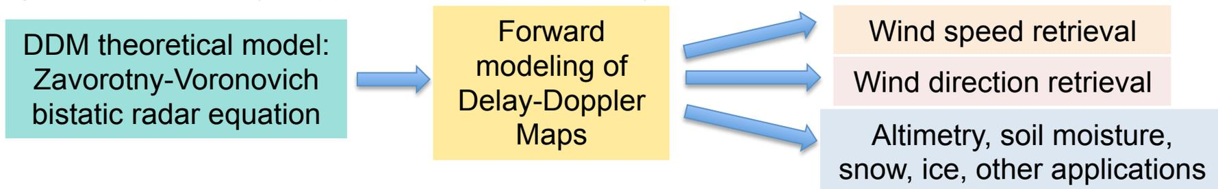
This model has proven successful in aircraft GNSS reflection experiments. Currently it is used to interpret data from recent space-based TechDemoSat-1 experiment simulations for future satellite GNSS reflection missions such as CYGNSS mission and others.
