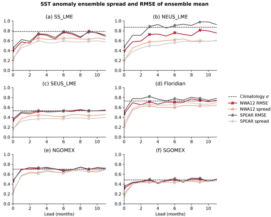
**Figure 9.** RMSE of NWA12 and SPEAR ensemble mean SST anomaly forecasts (dark red and gray, respectively), spread of the model ensemble members (light red and gray), and standard deviation of the observed anomalies (dashed black line). Letter markers on the lines mark whether the line is for NWA12 (N) or SPEAR (S).
