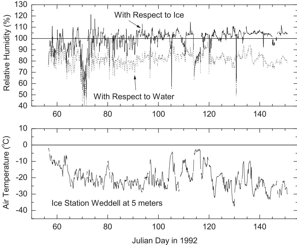
**Figure 4.** As in Figure 1, except these data come from a platinum resistance thermometer and a cooled-mirror dew-point hygrometer operated for almost four months on Ice Station Weddell in the Antarctic.
